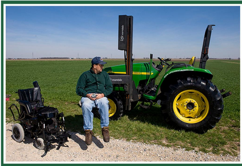
Automated lift for tractor cab access
